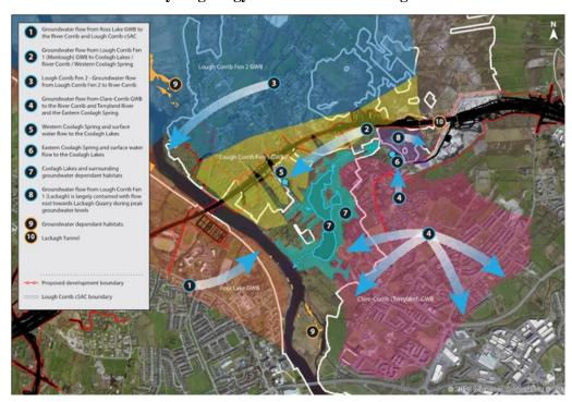
Plate 3: Generalised hydrogeology interactions with Lough Corrib cSAC
